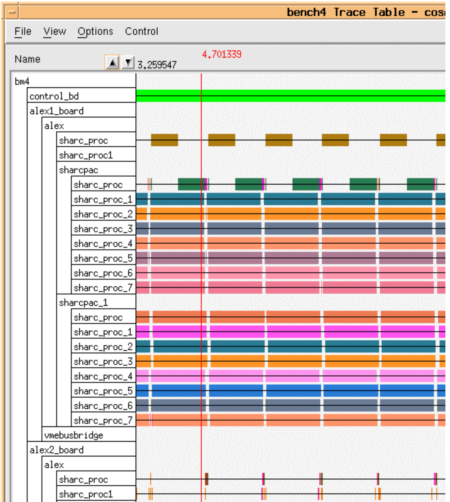
Figure 4 - 5: GEDAE™ Processor Table used when mapping software graph to the graphical hardware description
